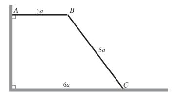
Two uniform rods AB and BC are smoothly jointed at B and rest in equilibrium with C on a rough horizontal floor and with A against a rough vertical wall. The rod AB is horizontal and the rods are in a vertical plane perpendicular to the wall. The rod AB has mass 3m and length 3a, the rod BC has mass 5m and length 5a, and C is at a distance 6a from the wall (see diagram). Show that the normal reaction exerted by the floor on the rod BC at C has magnitude  $\frac{13}{2}mg$ .
